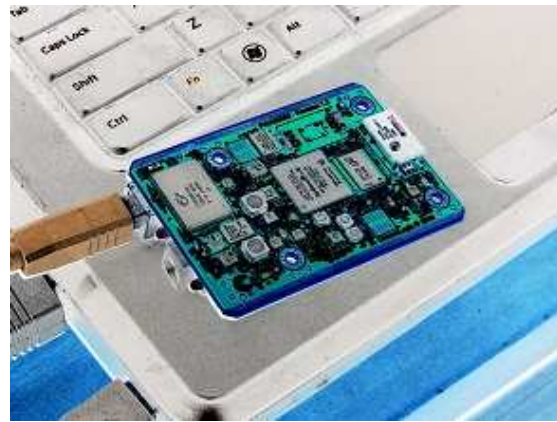
Figure 4 FPGA board, 28 Subleq processors with allocated 2 Kb per processor
